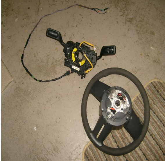
Clockspring and steering wheel. Next picture shows the 4 leads and where they attach to the J1 or J3 plugs.
