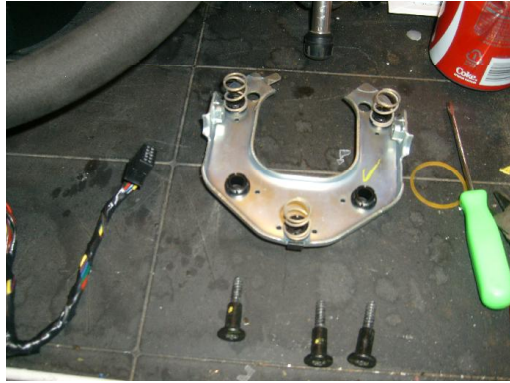
Plate shown removed with bolts and springs.
