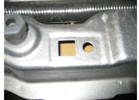
Top of radiator support has holes for mount tabs for both brackets
