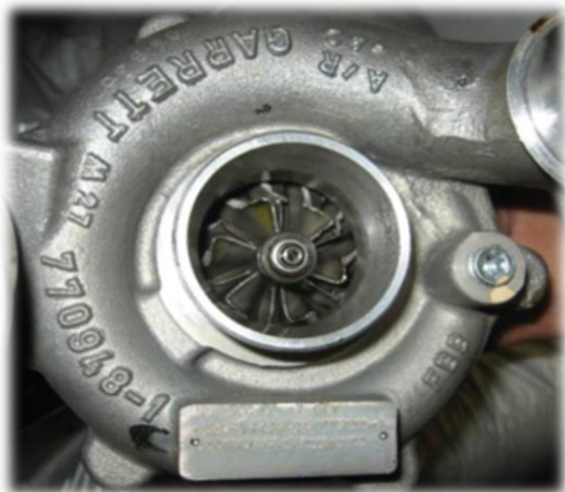
Figure 14: Compressor Blade Damage from Overspeed Event
