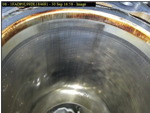
Figure 2: Scored Bore Walls
