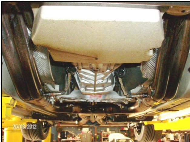
Figure 22: Long Tube Headers - Catalyst Delete and "X" pipe
