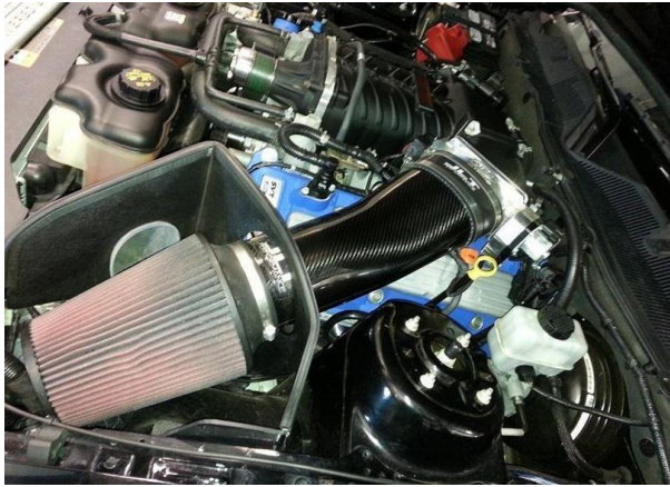
Figure 28: GT500 Aftermarket Air Filter, Inlet Tube, Throttle Body & Supercharger
