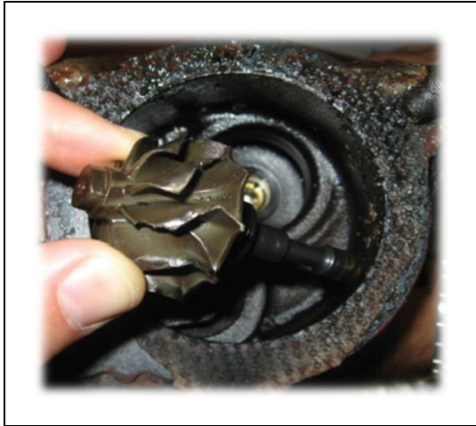
Figure 13: Compressor Blade Damage from Overspeed Event
