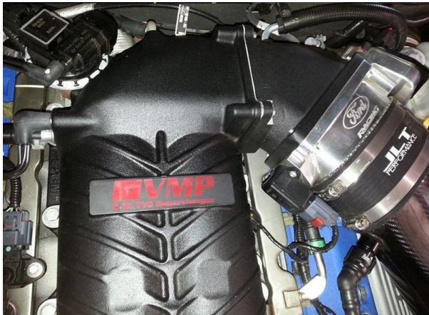
Figure 29: GT500 Aftermarket Supercharger & Throttle Body
