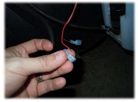
47. Strip the wires coming from the light assembly and attach corresponding crimp plugs to the wires.
