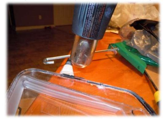
31. Test fit the headlight cover. Remove additional glue as necessary with the heat gun. Check that the tabs will reengage, use the heat gun to reshape them as necessary.
