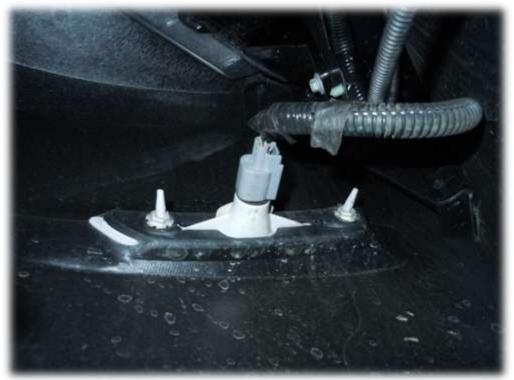
8. Remove or unplug the ambient air temperature sensor in the front valence.
