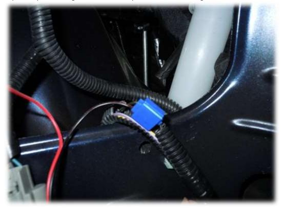
46. Take one male and one female crimp plug and attach it to the free ends of the lead wires.
