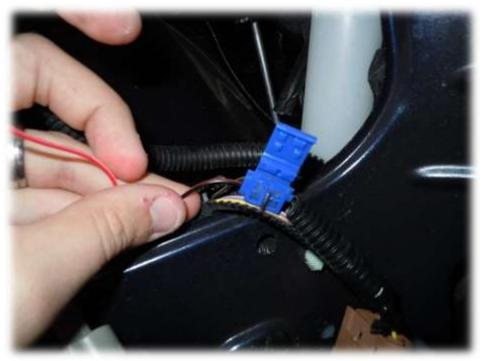
44. Using the multimeter, check for continuity on the other end of the red wire and the purple/white wire by using the terminal on the side marker light. If there isn't continuity, redo the connection and check again.
