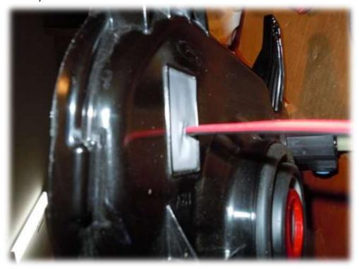
29. Insert the inner cover back into the housing. Route the wiring through the hole in the seal. Route the wire behind the deflector and pull the slack out the back of the housing.
