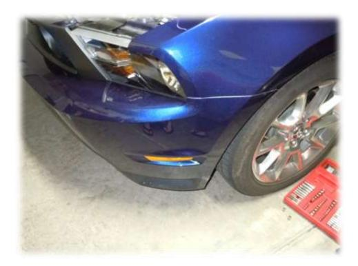
11. Remove the two 8mm bolts from the top of the grill, lift the cover off the tabs beside the bolts and remove the bumper cover.
