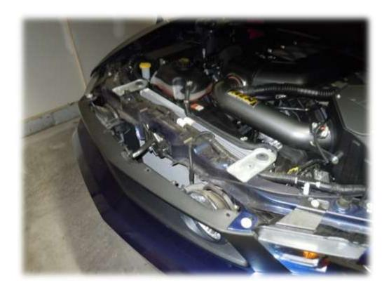
3. Remove the 4 splash shield screws (2 each side) with the 7mm socket.
