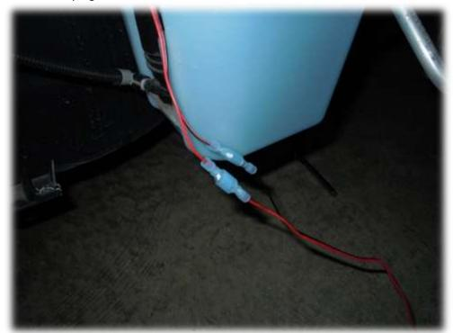
49. Turn on the parking lamp switch to check the electrical connection. If the lamp does not turn on, turn off the switch and proceed to check your crimps for continuity with the wire. If the connections are sound, try the switch again until the light turns on.
