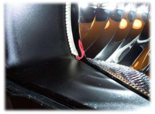
30. Remove any sealant from the headlamp cover with a screwdriver and the heat gun.
