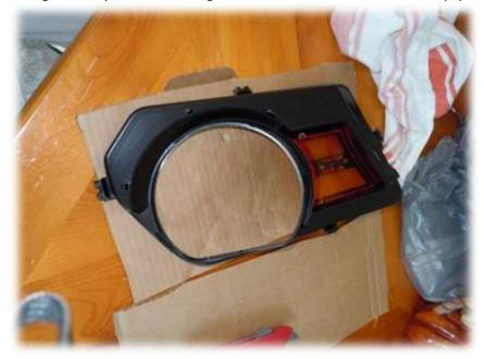
23. Remove the Oracle Halo unit from its wrapping. Test the LEDs using a 12 V power source. If faulty contact American Muscle or the manufacturer. Line up the ring with the back edge of the cover.
