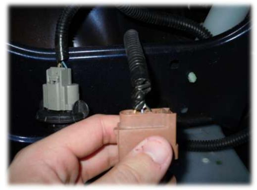
38. Use a knife, scissors, or a pair of snips to remove a portion of the wire routing.
