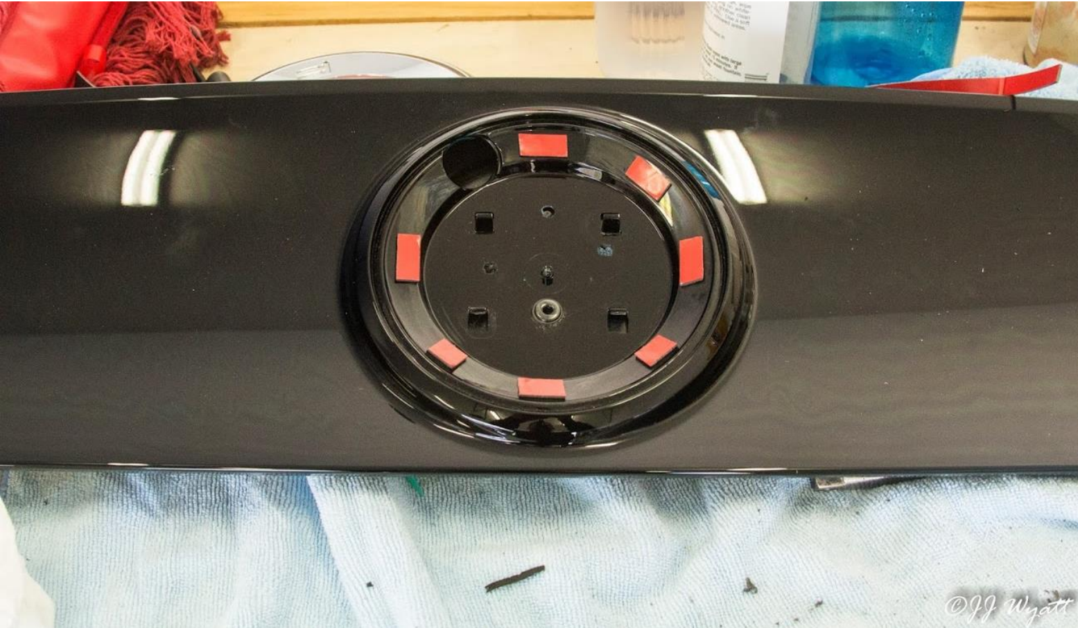
Here I used small strips of 3M to help those four "C" clips hold the faux cap in place.
