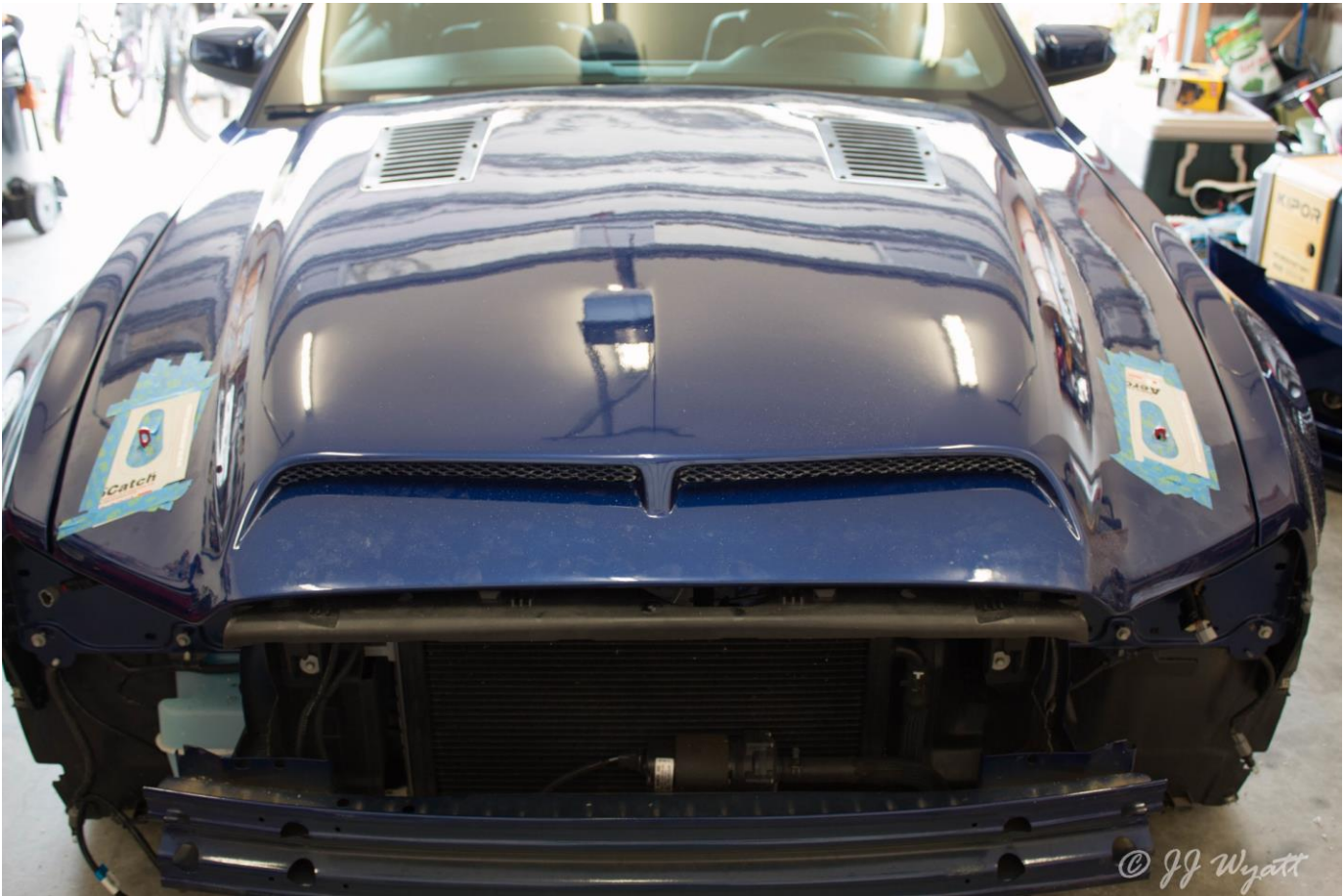
Get a suitable hood support and cut it out. (I used a cutting wheel to take out most of it, but stayed away from the line. Then I used a sanding wheel to clean it up.)
