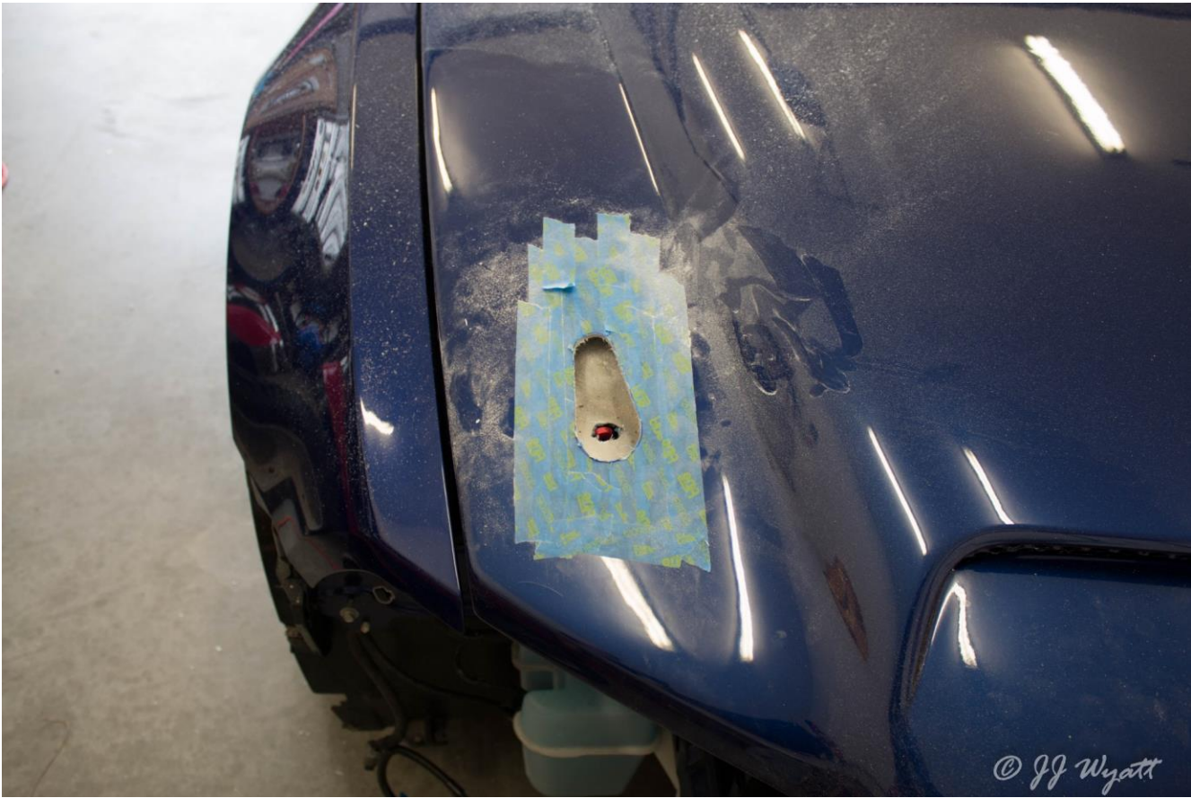
For the bottom I used a carbide bit. Looking from the top I cut from the bottom. Then I cleaned it up with a sanding wheel.
