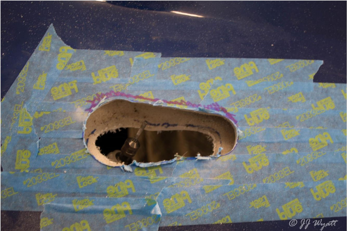
For the bottom I used a carbide bit. Looking from the top I cut from the bottom. Then I cleaned it up with a sanding wheel.
