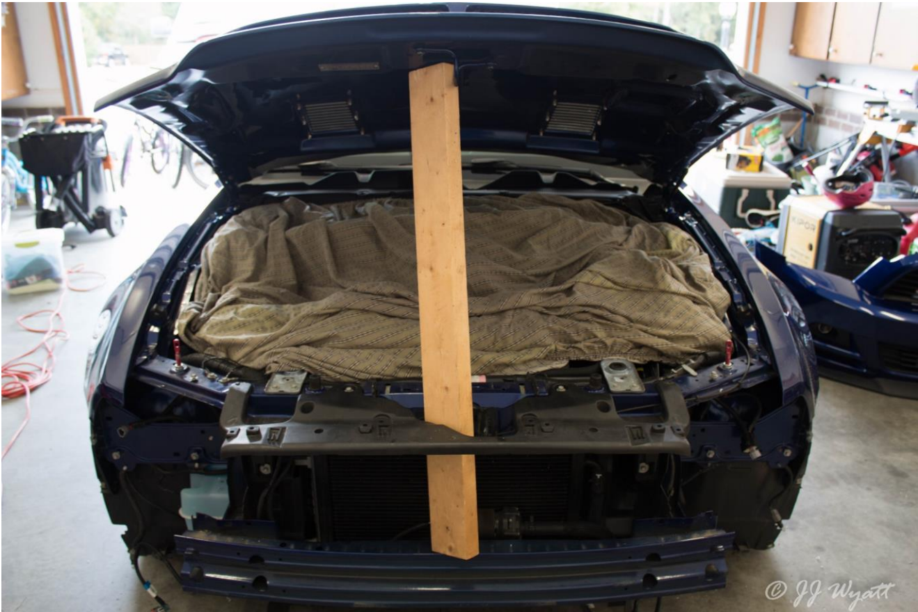
Get a suitable hood support and cut it out. (I used a cutting wheel to take out most of it, but stayed away from the line. Then I used a sanding wheel to clean it up.)
