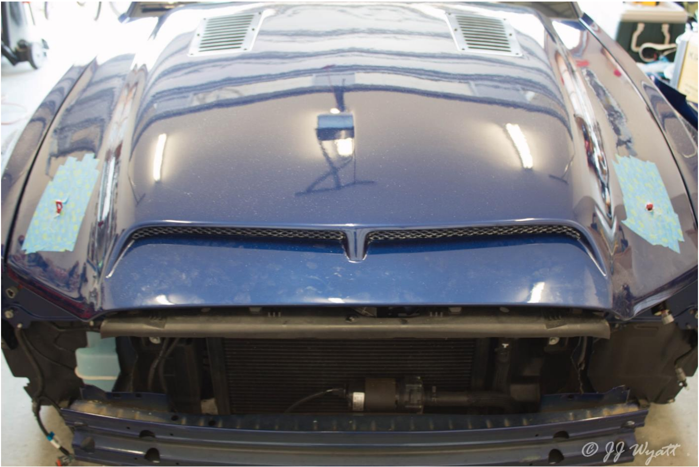
Now align the templates and tape them in place. (Once aligned I used a sharpie and traced the inside.)
