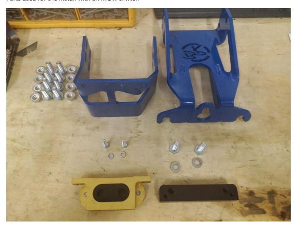
With the MGW you will reuse the two post bracket. Attach the two post bracket to the Blowfish adapter bracket.
