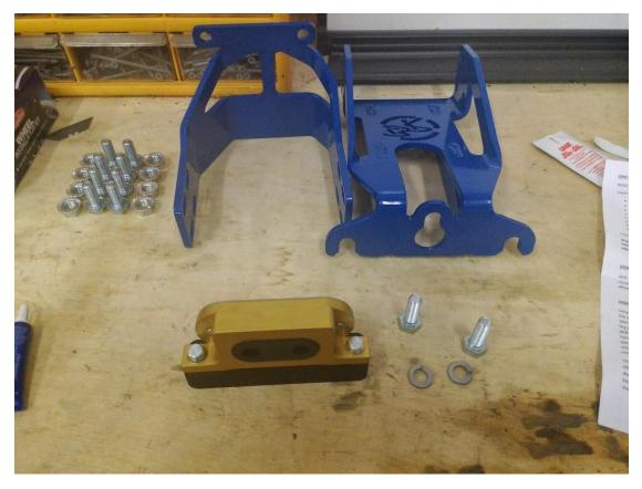
The MGW two post bracket will be re-installed, but you would install it upside down so the Blowfish adapter bracket is facing down.
