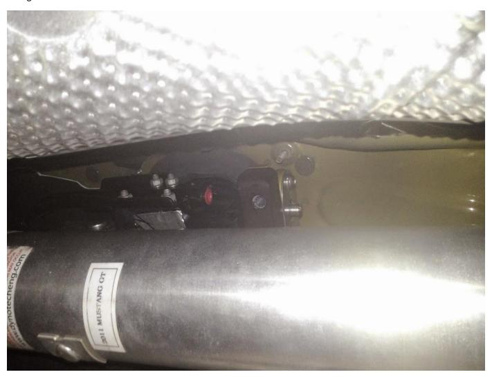
The instruction now call for you to install the lower bracket. If you have an X-Pipe I suggest that you install the upper bracket first according to the instructions and slide it towards the rear of the vehicle out of the way then install the lower bracket. I had to remove the lower bracket and do this. The "X" is right in the way of being able to rotate the upper bracket around the Drive Shaft.
