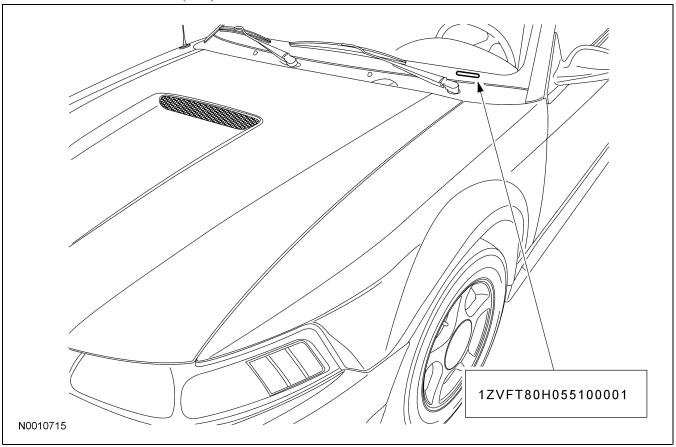
The vehicle identification number (VIN) is a 17-digit alphanumeric code. The VIN is stamped on a metal tab riveted to the instrument panel, top upper left of the dash. The VIN number is also found on the vehicle certification (VC) label.
