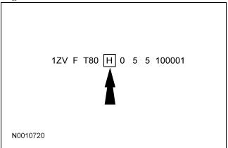
The 8th VIN position is the engine displacement and number of cylinders code.
