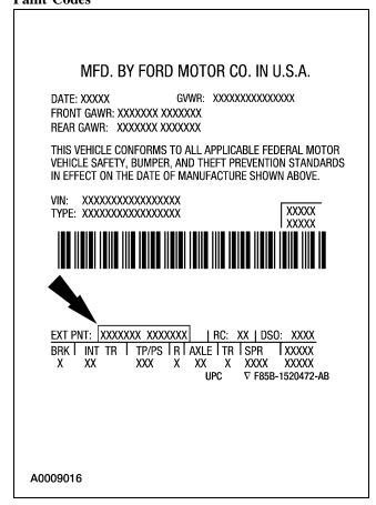
The 1st set of paint code letters/numbers listed indicate the vehicle primary body color. The 2nd set of paint code letters/numbers listed (if applicable) indicate a 2-tone or accent body color. All colors are base coat/clear coat.
