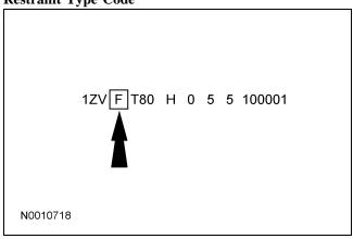
The 4th VIN position is the vehicle restraint system type code.
