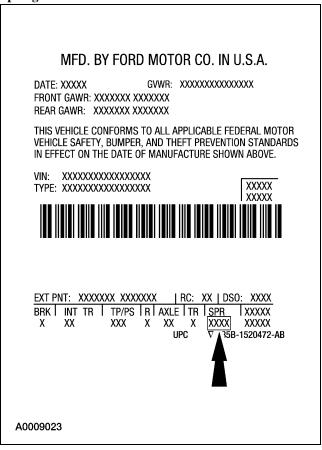
The spring code portion of the vehicle certification (VC) label identifies both the front and rear springs. The 1st letter/number indicates the front spring code. The 2nd letter/number indicates the rear spring code.
