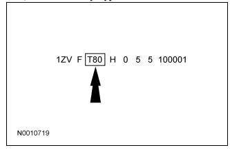
Positions 5 through 7 indicate vehicle line, series and body type.
