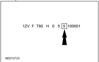
The 11th VIN position is the assembly plant code.
